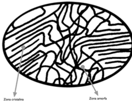
Crystalline areas allow the high density polyethylene a higher resistance, for different thermal cycles, recovering its shape and maintaining its properties along the years.
