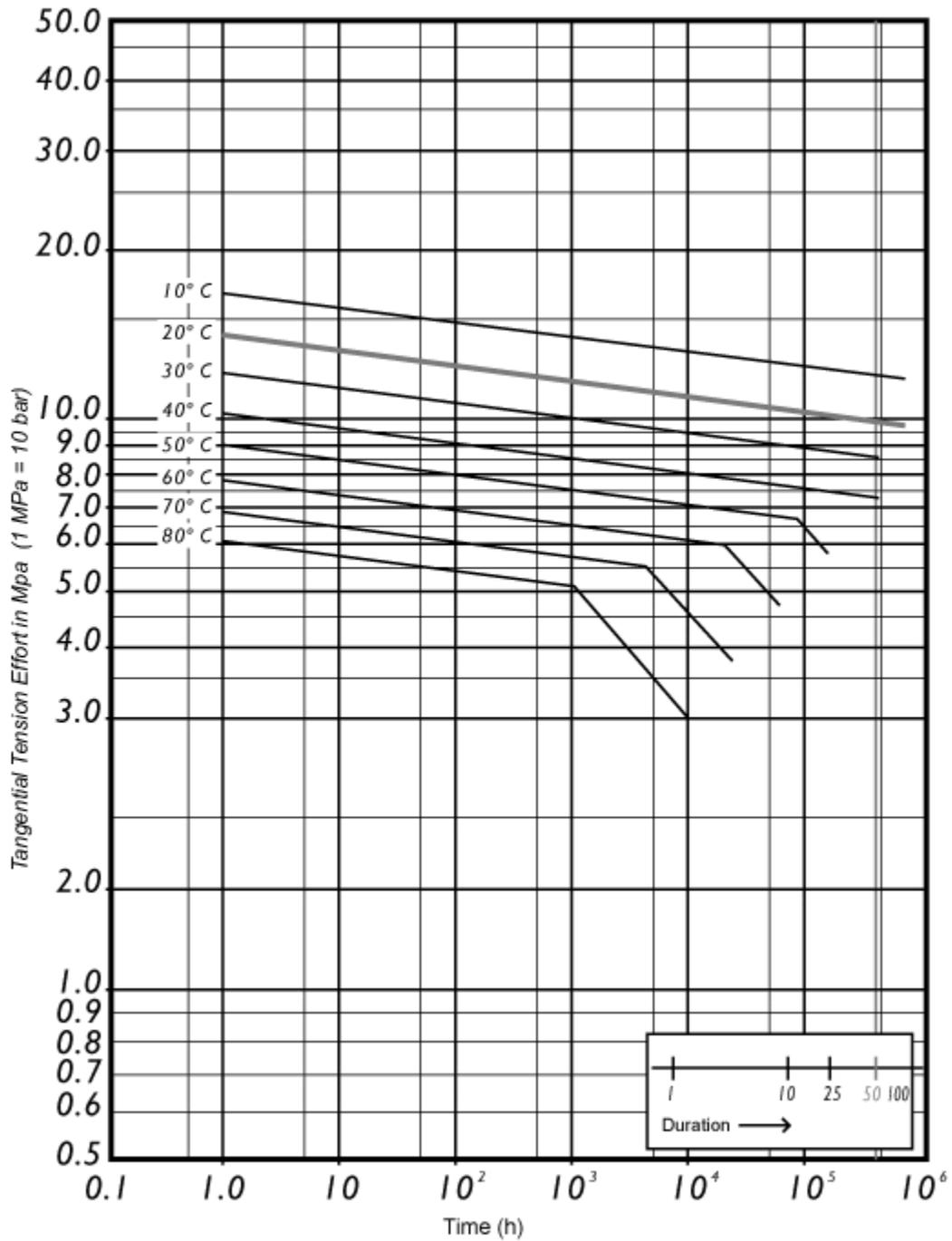
Fig. 4 - Regression curves PE100 (Source DIN 8074)
