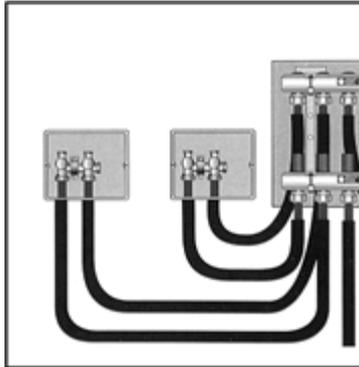
Installation example: FILTERMO with FILFLEX
