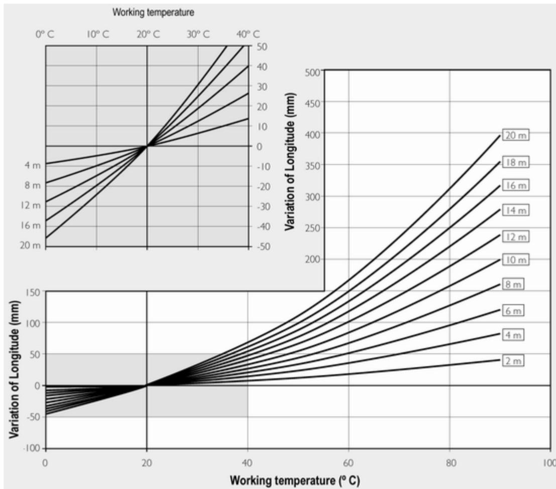
Graph 2-Linear thermal expansions of the Crosslinked Polyethylene pipes, considering Ambient Temp=20°C
