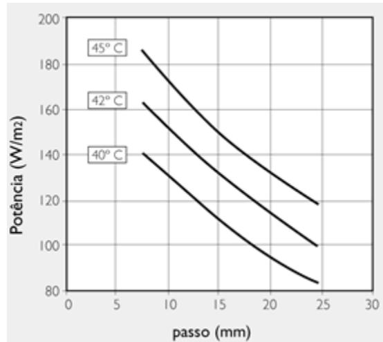
Graph 7 - Values of power finish of heating in function of the applied step and of the temperature of going of the water, for ceramic pavements and ambient temperature of 19°C
