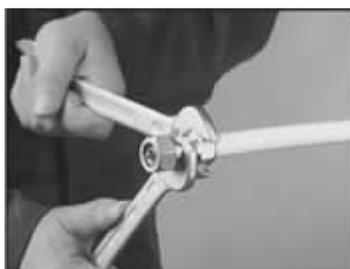
Fig 12. fitting adjustment
