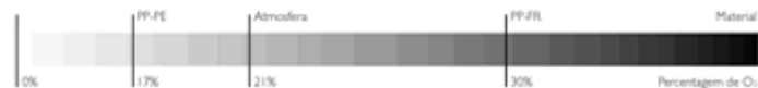
Fig. 2—percentage of necessary oxygen to maintain the flame lit in a combustion
