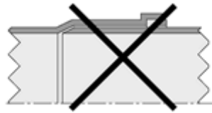
Fig. 5 - installation of SANIFIL not allowing the absorption of thermal expansions.
