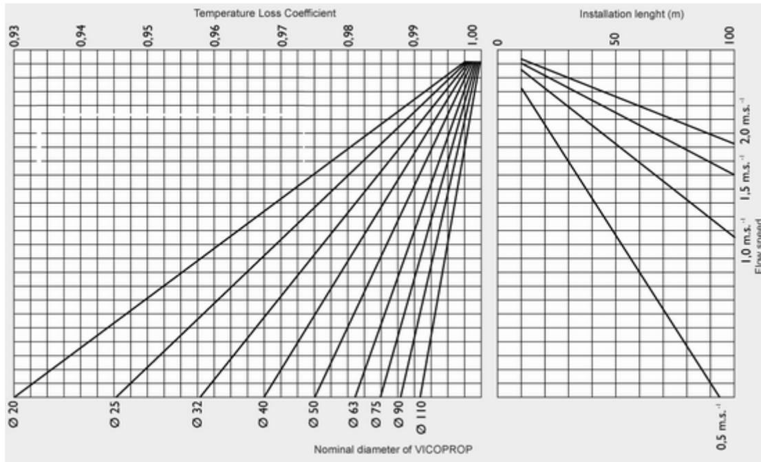
Graph 7 - VICOPROP PN10 temperature losses coefficient (water transport temperature of  $50^{\circ}\text{C}$  and external temperature of  $20^{\circ}\text{C}$ )
