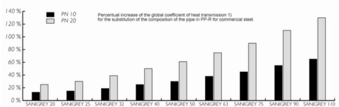
Graph 6-Comparison of the global coefficient of transfer of heat 1) considering the composition of a pipe geometrically and dimensionally similar to the VICOPROP pipe, but composed by commercial steel.
