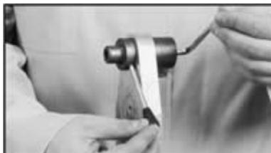
Image 7 - Connection of the socket welder
