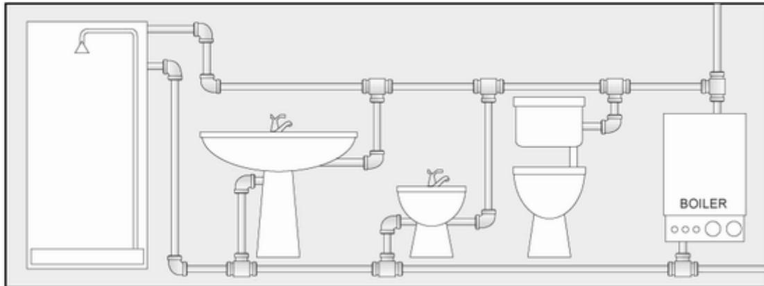
Fig. 4- Sanitary installation with VICOPROP system
