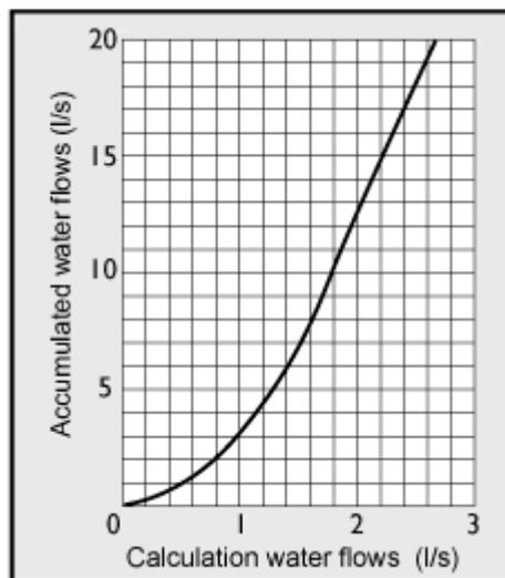
Graph 8-Calculation water flows in function of the water flows accumulated for a level of medium comfort
